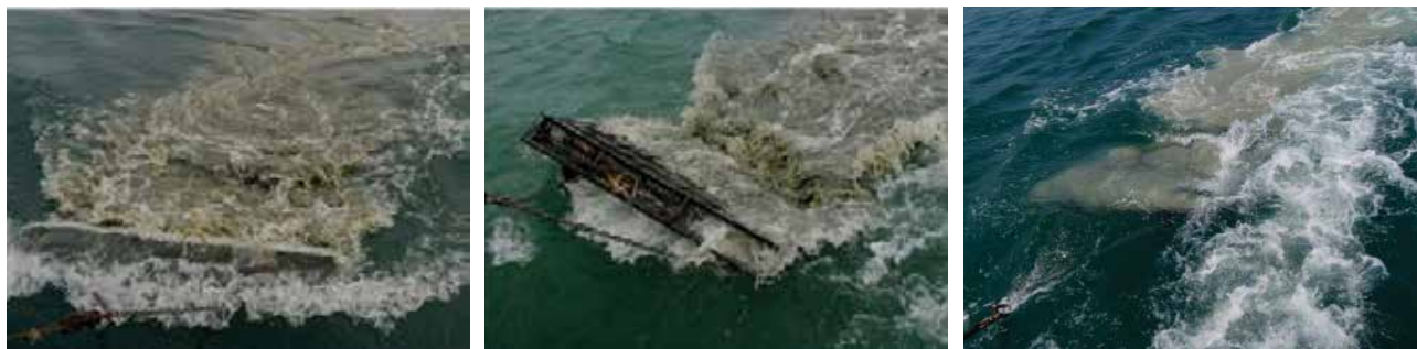
Fig. 5. Re-suspended sediment spreading at the sea surface while the dredge is being hauled
