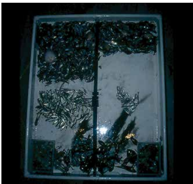
Fig. 4b. The difference in catches and by-catches when using the panel (right side of the tray) compared to a conventional control codend (left side of the tray).
