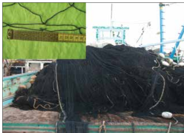
Fig. 3. Polyamide gillnet stored on board tuna fishing vessel at Karachi. Inset: stretched mesh.
